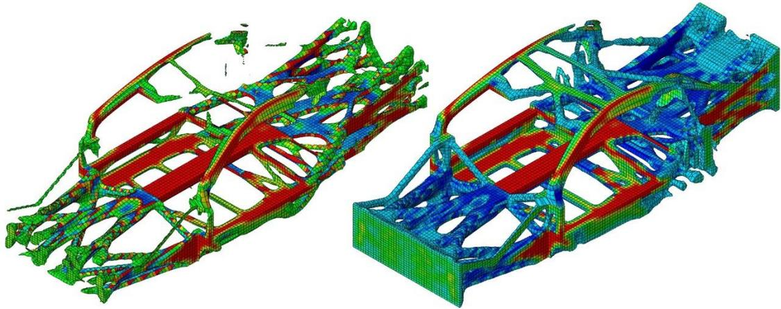
**Figure 13: topology optimisation result, for as minimum element density set respectively to a value of 0.5 and to a value of 0.25**
