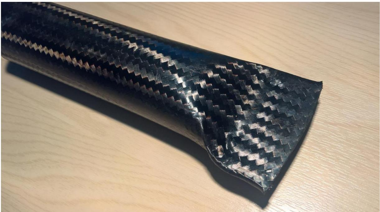
**Figure 35. Braided thermoplastic CFC tube with subsequent end-flattened geometry**
