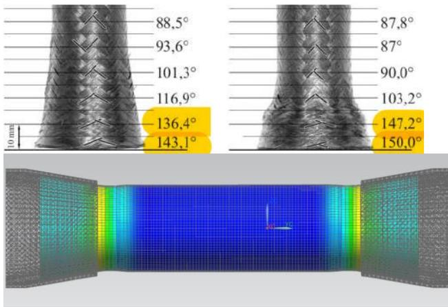
Figure 22: Top: flange angle and influence on space and weight. Bottom left: influence of swaging on fibre orientation [11]. Bottom right: stress concentration at the tip of the fittings.
