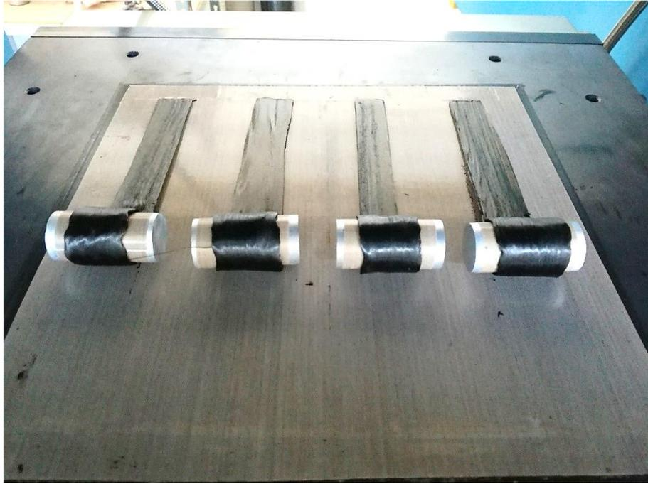
**Figure 50: UD laminates wrapped around 25mm diameters**
