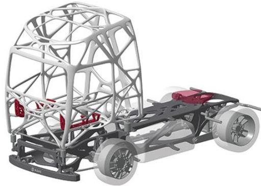
**Figure 1: Three of the four above images come from the EDAG, who are feeding the trend of optimised 3D printing with substantial use of the software package Optistruct™, from Altair.**
