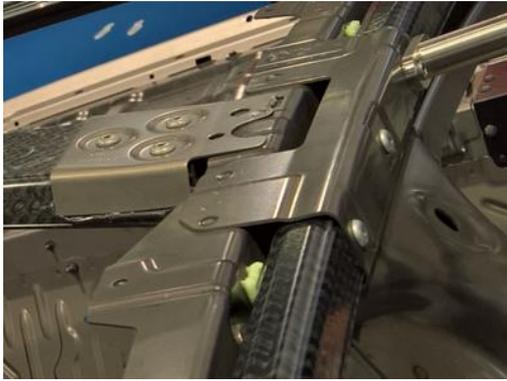
**Figure 37. Metal over-plate joints onto CFRP structures in BMW G11/ G12 (7 series), JEC World 2017**
