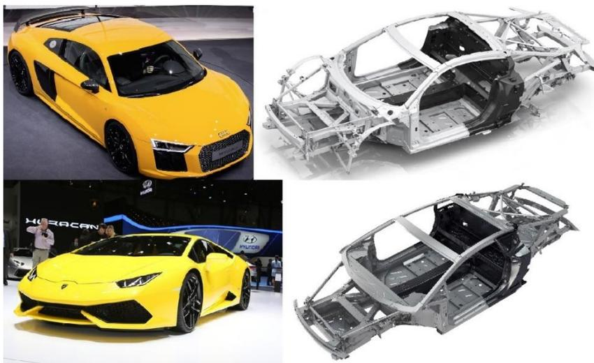
**Figure 9: Audi R8 and Lamborghini Huracan. Both structures are made of aluminium and carbon fibre composites. The platform is the same, but the upper part differs due to exterior aspect.**
