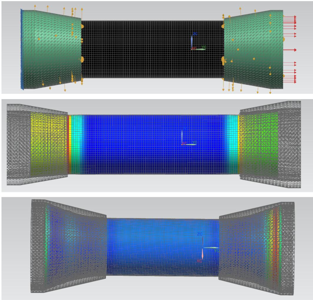
**Figure 42: Top: tensile FEA model. Middle: tensile FEA result. The scale is relative, highlighting stress concentration at the edge of the fitting. Bottom: Compression result on a greater swaging angle. Relative scale**
