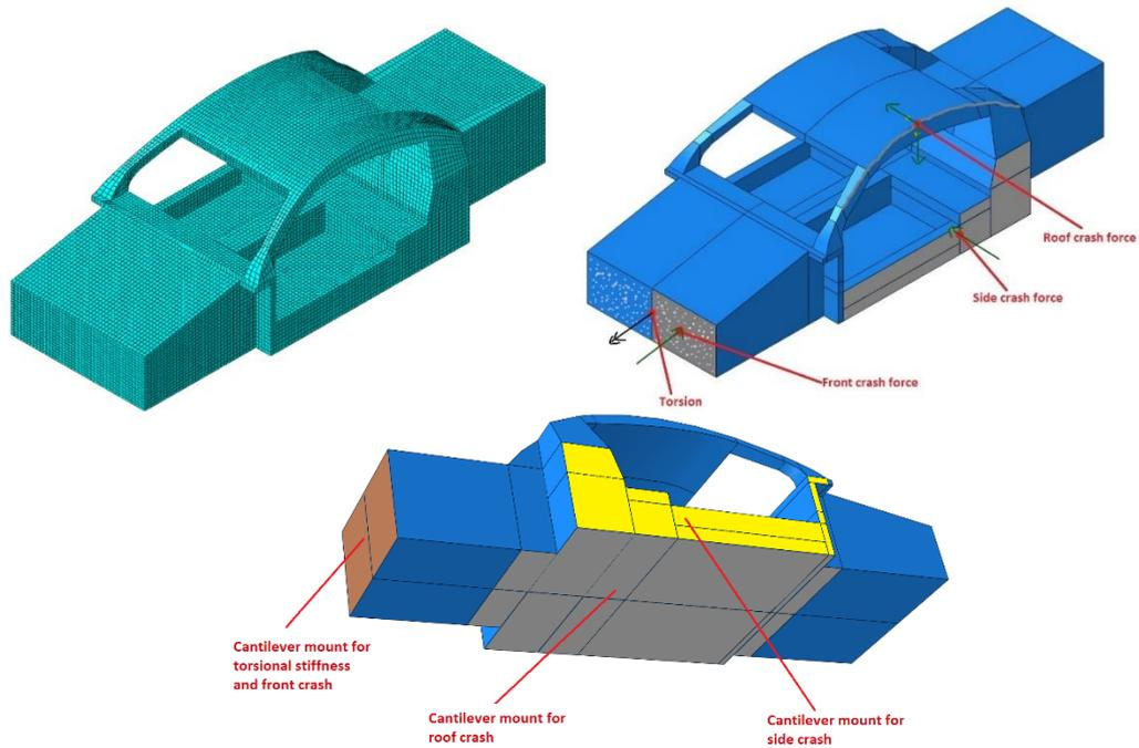
**Figure 12: Top left: the number of elements of the model is around 90,000, determine by convergence study. The geometry of the model is divided in areas where the boundary conditions are applied.**
