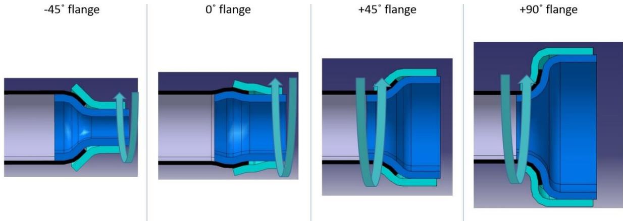
The hot end of the TP matrix braided tube is formed onto the threaded mandrel, then the threaded hat is screwed to the mandrel, resulting in clamping the tube
