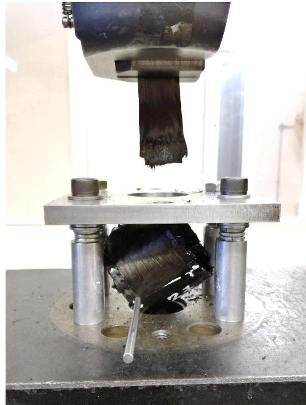
**Figure 56: the laminate, respectively  $\pm 45$  and UD, has failed before the bonding interface**
