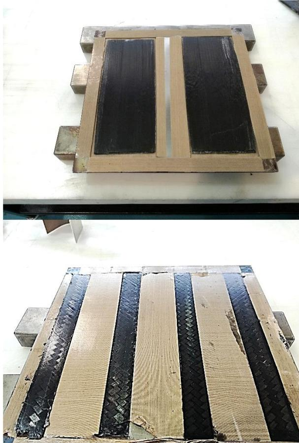
Figure 49: Organosheets. On the left: UD laminates, before being cut in 25mm wide strips. On the right:  $\pm 45^\circ$  laminates, 25mm wide.
