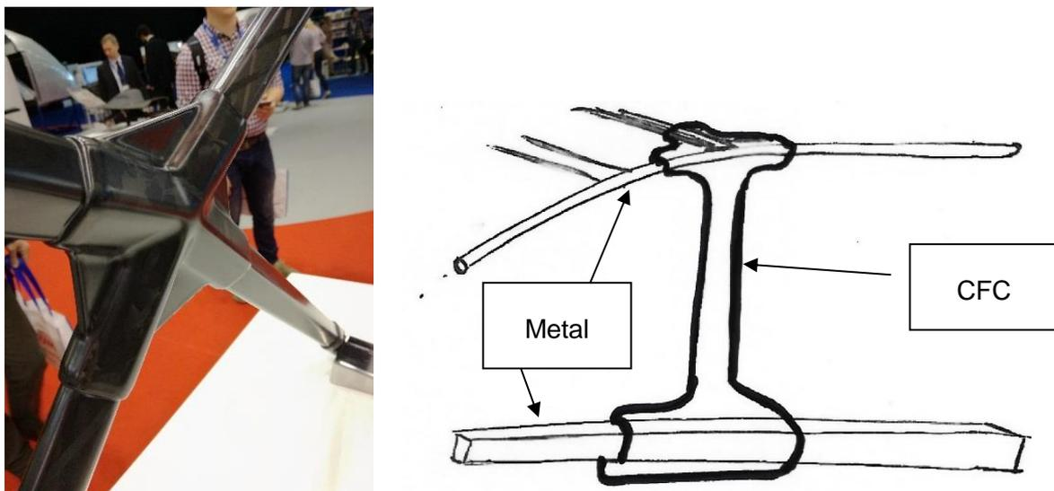
Figure 23: Left: Secar for Audi R8, four pultruded tubes are assembled by over moulded SMC node. Right: B-pillar + composite-to-metal joint as a single part
