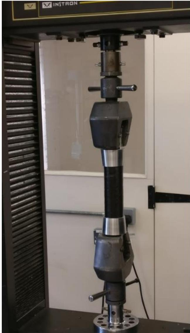
**Figure 45: Final assembled coupon, and tensile test apparatus**
