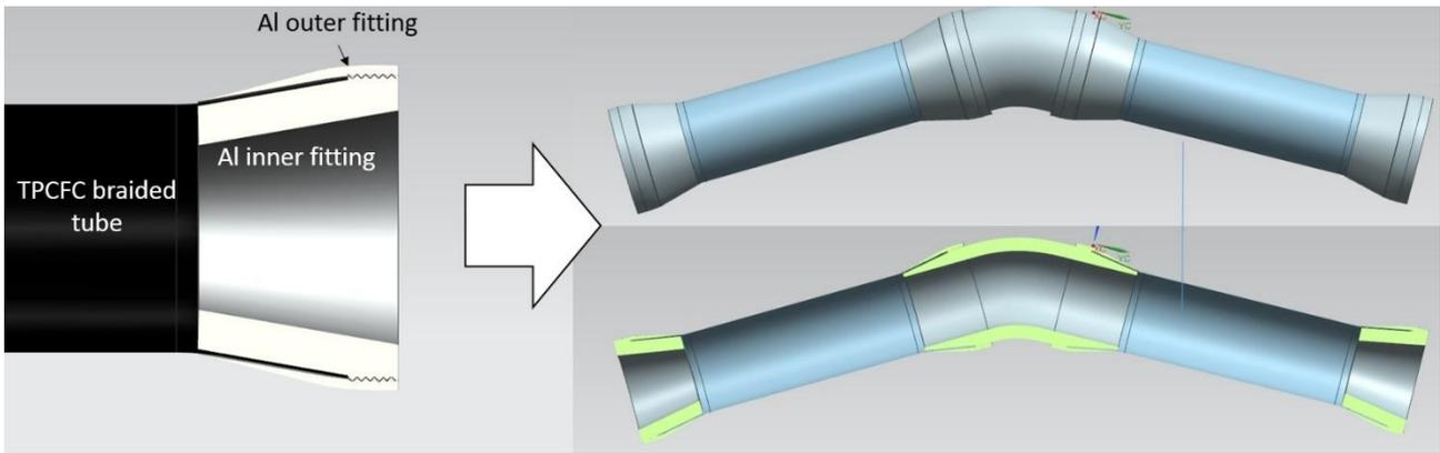
**Figure 21: TP carbon tube swaging. Threaded metal-to-metal connection**
