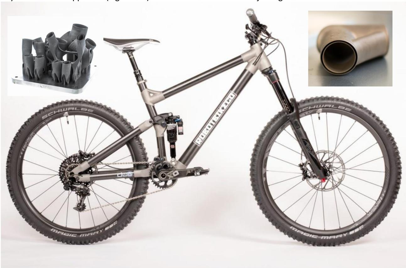
Figure 19: Robot Bike™, thermosetting composite tubes and titanium nodes. The frame alone costs 4400£. The cycle time is 48h. Source: RobotBike.co
