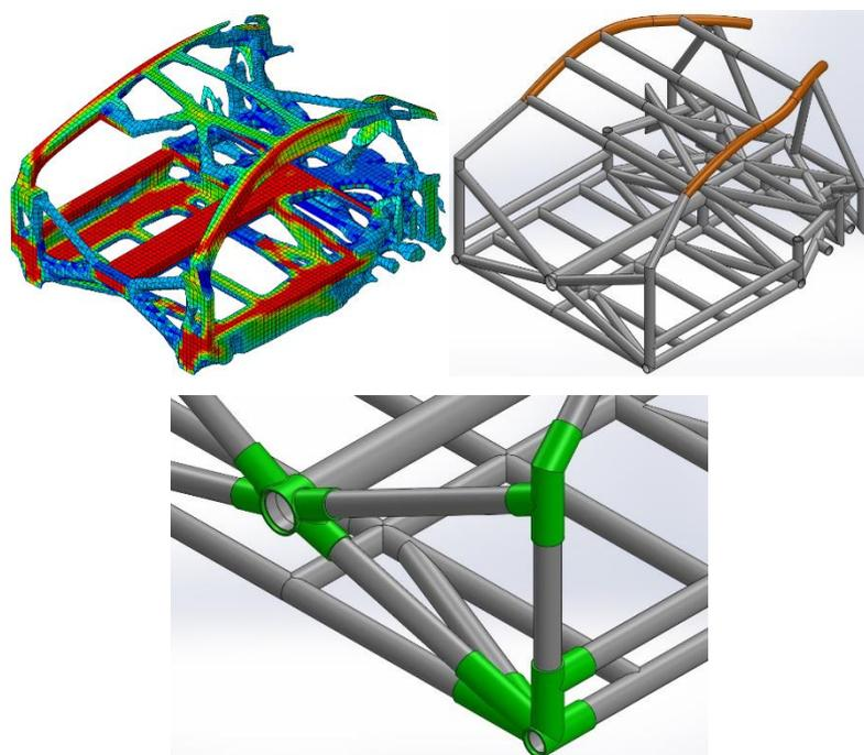
**Figure 16: from optimised cockpit, to concept 2, to corresponding zoom on nodes. Three different manufacturing processes are highlighted, in three different colours**
