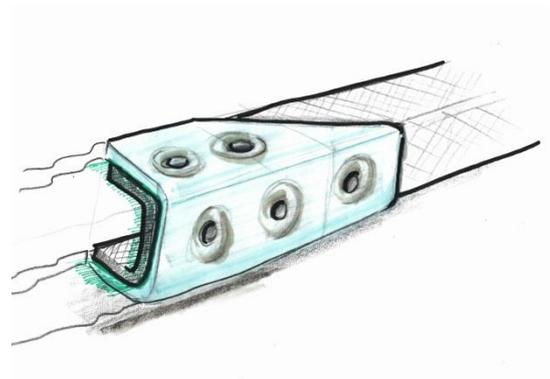
**Figure 40 Schematic sketch of dimple-joint concept applied to C-Shape CFC framework element to metallic end-node structure**
