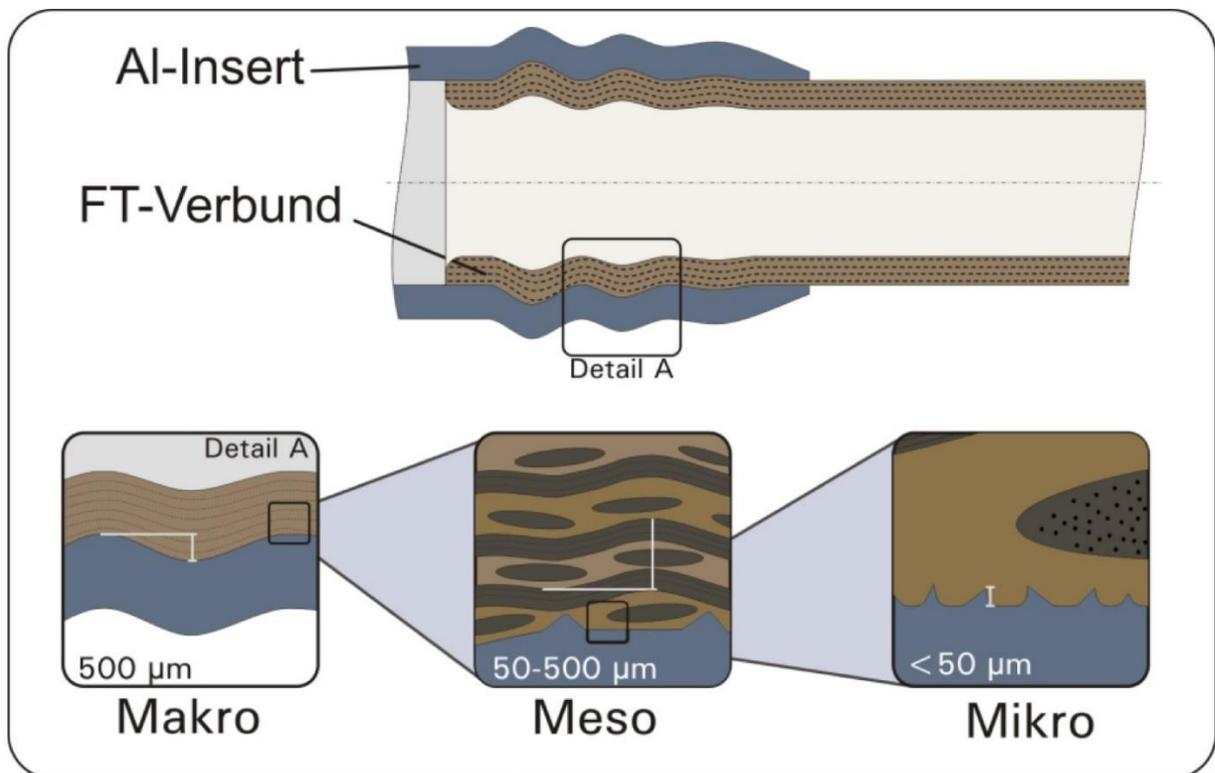
**Figure 20: TU Dresden's multi scale approach of joining. The macro scale being the essential benefit to traditional adhesion joints. Source: TU Dresden internal report**
