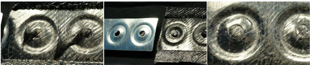
**Figure 65 - "dimple-down" specimen** **Figure 66 - "dimple-up" specimen** **Figure 67 - "capped" dimple after exhibiting failure of CFC material failure surfaces (metallic failure, exhibiting removal of where interlocked into metallic component, left, inverted from test polymer material from fibres in through-hole orientation to reveal joined faces) centre-most circular regions corresponding to through-hole in metallic plate**
