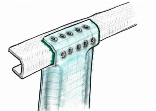
**Figure 39. Schematic sketch of dimple-joint concept applied to upper B-Pillar metallic/ CFC structure**
