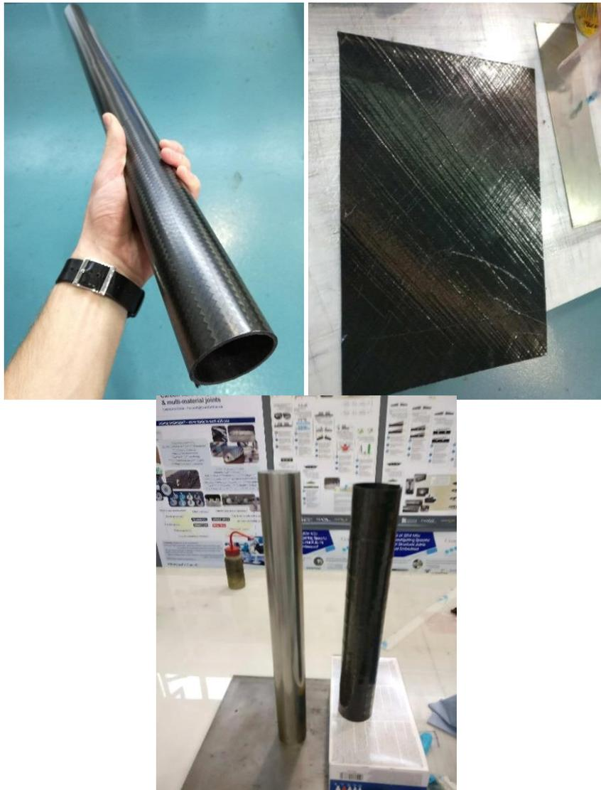
**Figure 43: Left: Dresden TU biaxial braided PA6 CFC tube. Middle: HS carbon fibres infused with L&L L-F610 reform able epoxy. Right: mandrel and tube formed from infused HS. The laminate is biaxial too, and the volume fraction is 50%**
