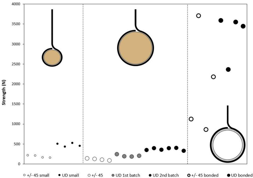
Figure 54: Strength results for all the wrapped samples manufactured. The three zones concern respectively configurations 1 and 2; 3 and 4; 5 and 6.
