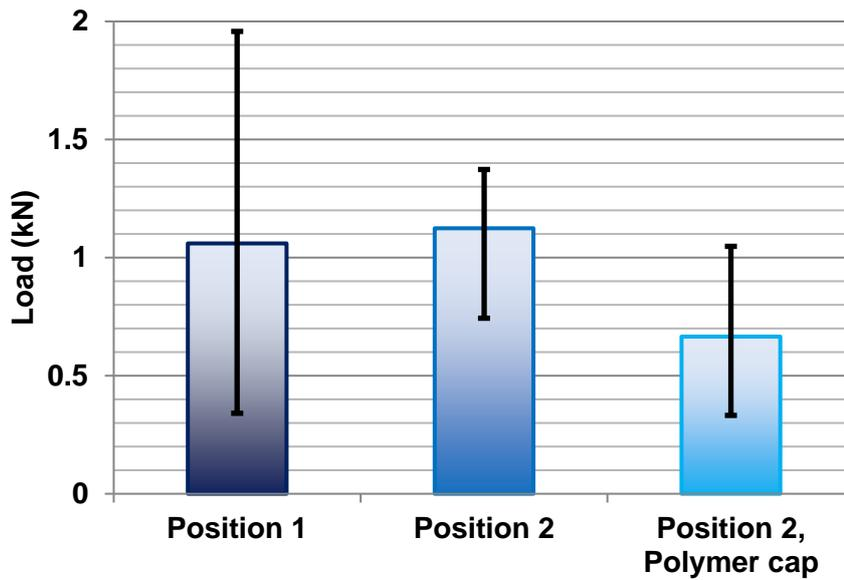
Figure 61 Mechanical testing results for metallic/ CFC dimple joint specimens
