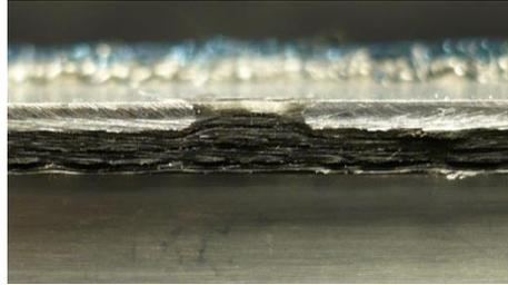
**Open hole in flat metallic sheet** Some degree of material flow into hole, estimate 20 to 30% filled
