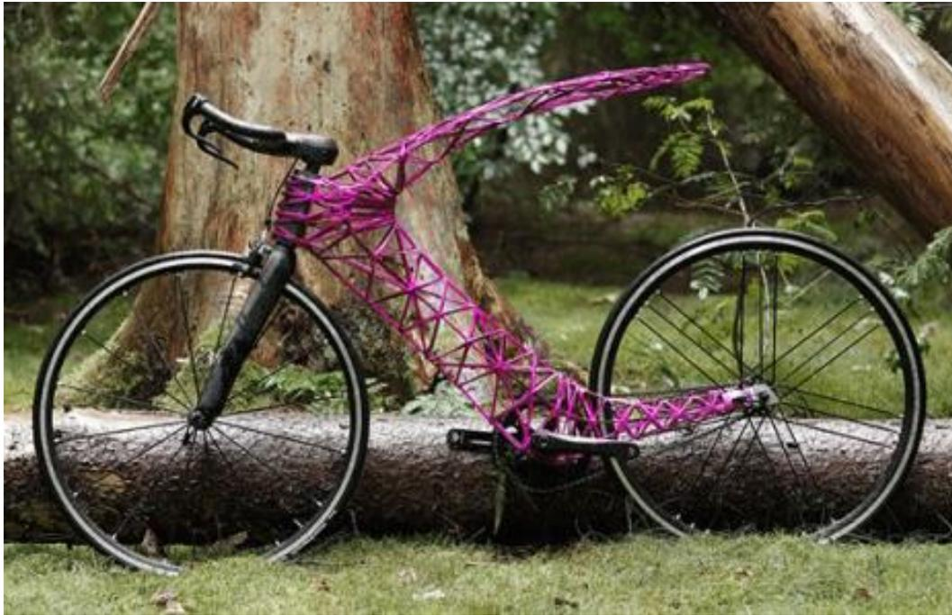
**Figure 2: The Cirkomp isogrid bike, a mix of bionic and geodesic shapes**
