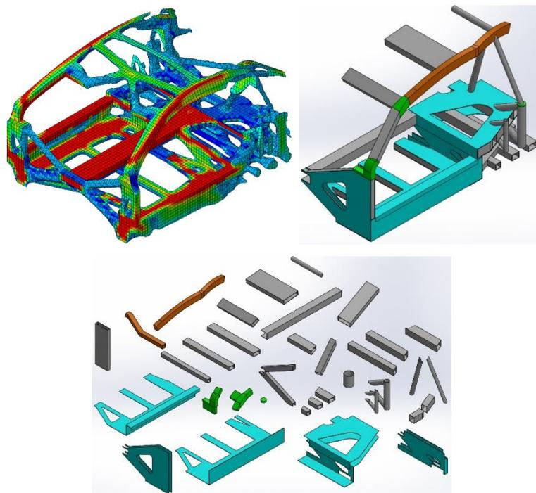
**Figure 15: from optimised cockpit, to concept 1 (half view), to corresponding exploded view. Four different manufacturing processes are highlighted, in four different colours**
