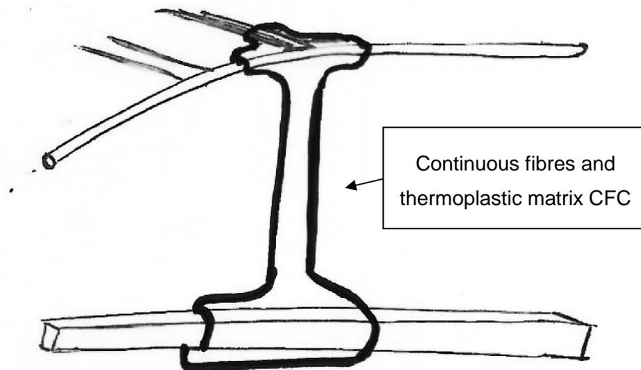
Figure 47: concept sketch of a CFC B-pillar attached to a framework via the deformation of its ends
