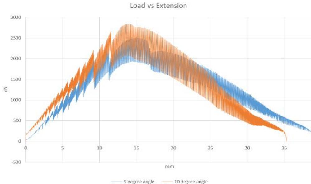
**Figure 46: tensile test results comparison between 5 degrees swaging angle coupon and 10 degrees swaging angle coupon**
