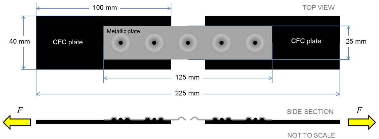
Figure 60. Mechanical test specimen configuration
