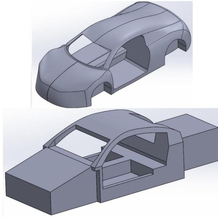
**Figure 10: CAD design zones for the case study of a revisited Audi R8. On the left, the design is conservative and follows the current envelop of the R8. On the right, a simplified design zone that allows faster computational time, and greater design freedom.**
