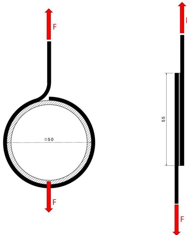
Figure 57: Configurations 5 and 6 (left) provide equal or greater strength than scaled single lap joint (right).
