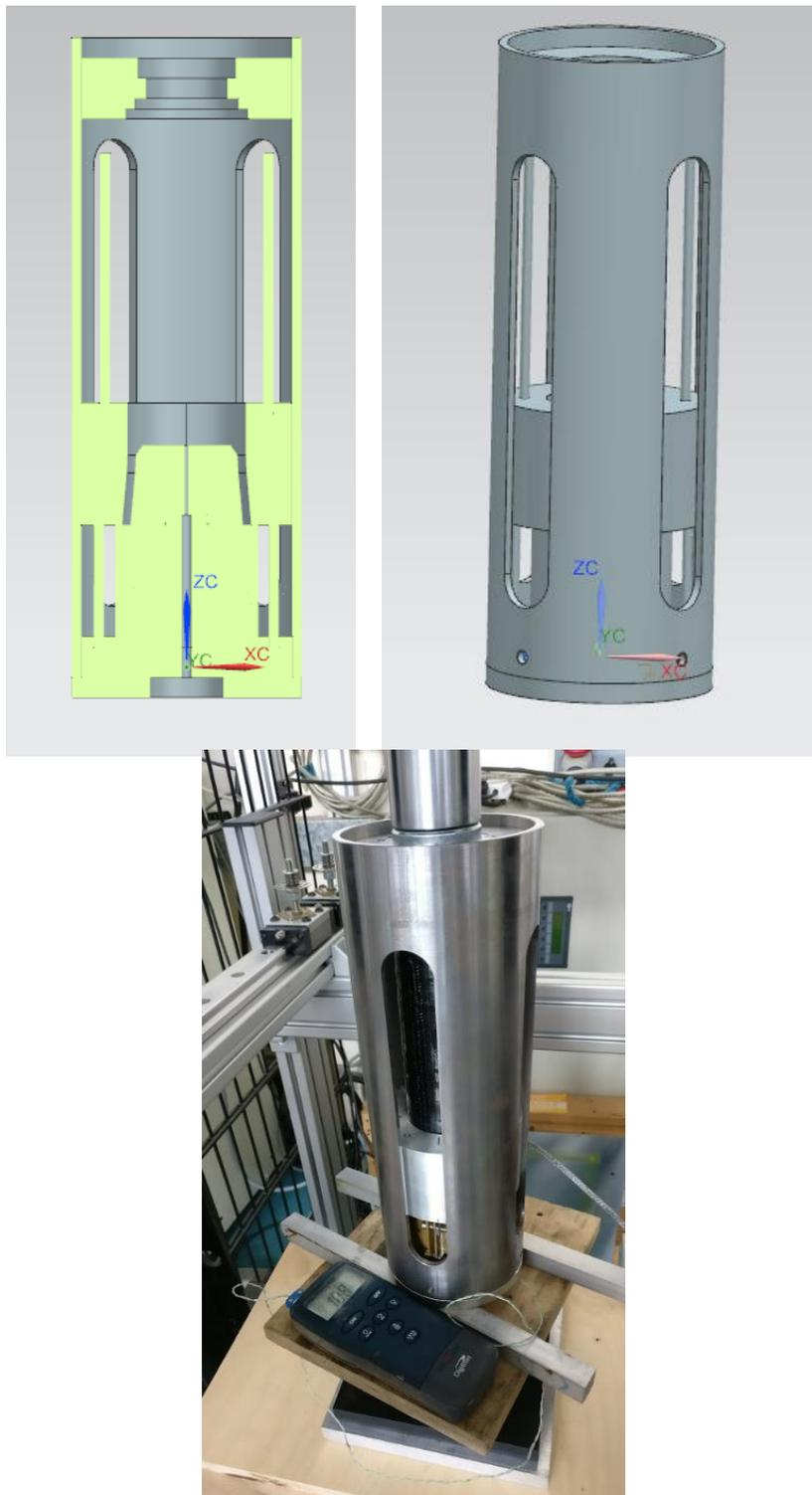
**Figure 44: Tooling assembly section view, side view, and manufactured part.**
