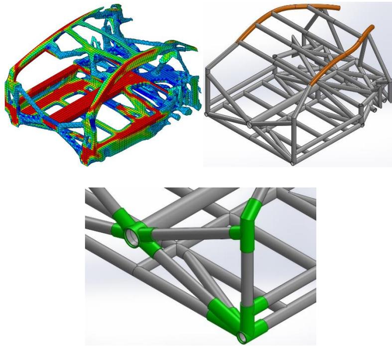
Figure 40: From optimised cockpit, to concept 2, to corresponding zoom on nodes. Three different manufacturing processes are highlighted, in three different colours.
