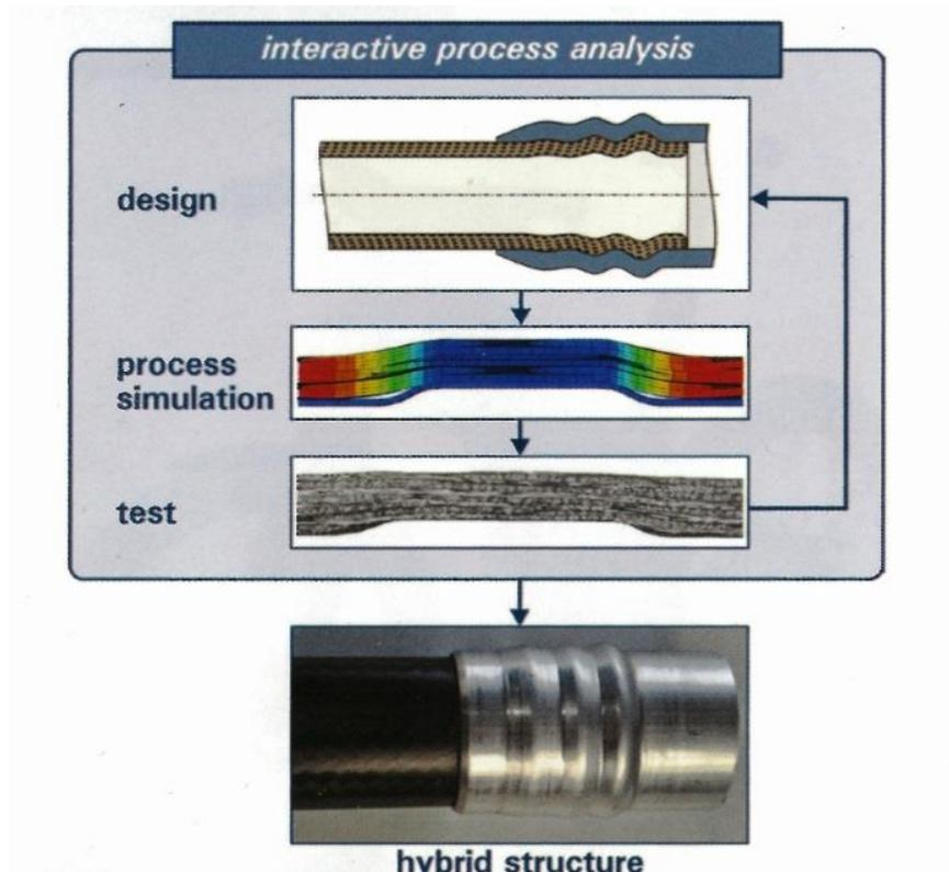
**Figure 31. - swaged metallic/ thermoformed CFC joint, courtesy of ILK TU**
