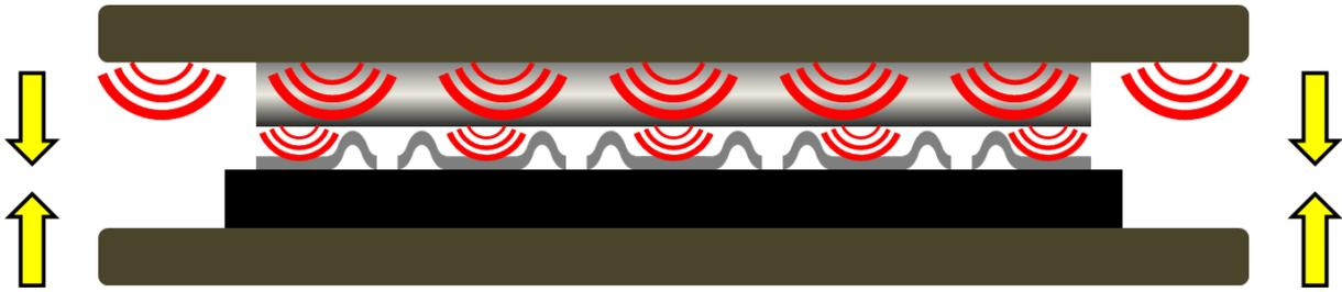
Figure 59. Dimple joint pressing arrangement (not to scale)
