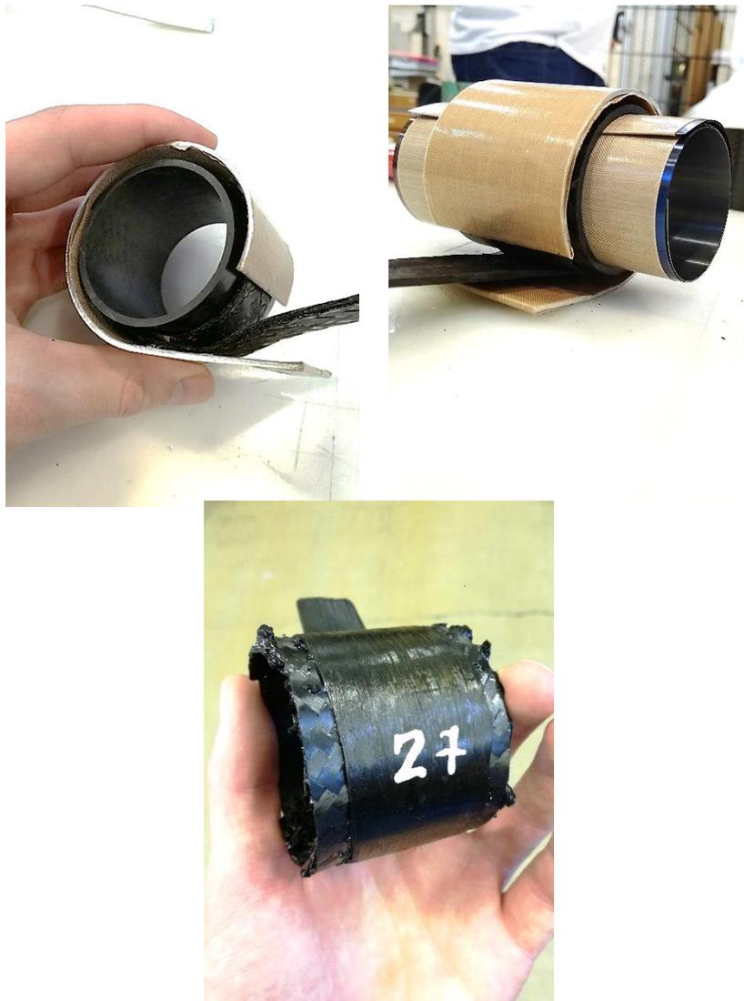
**Figure 52: Left: positioning of the tube and wrapped laminate in the outer mould. Middle: the inner spiral spring mould is added. Right: finished sample, after consolidation at 250°C and release. The pressure in the mould was sufficient to create an excess flash of resin on the sides of the tubes.**
