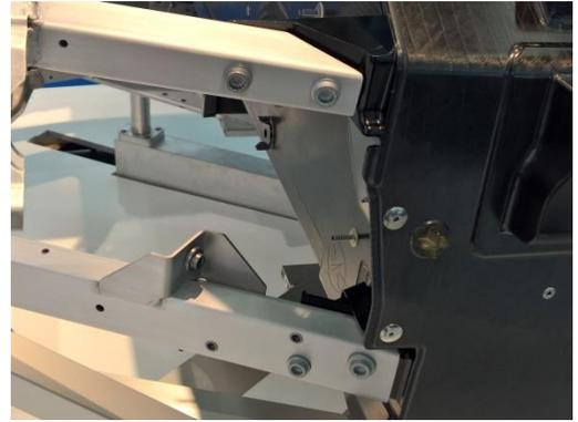
**Figure 38. Through-bolted multi-material joints in an Audi R8 rear chassis framework, JEC World 2017**
