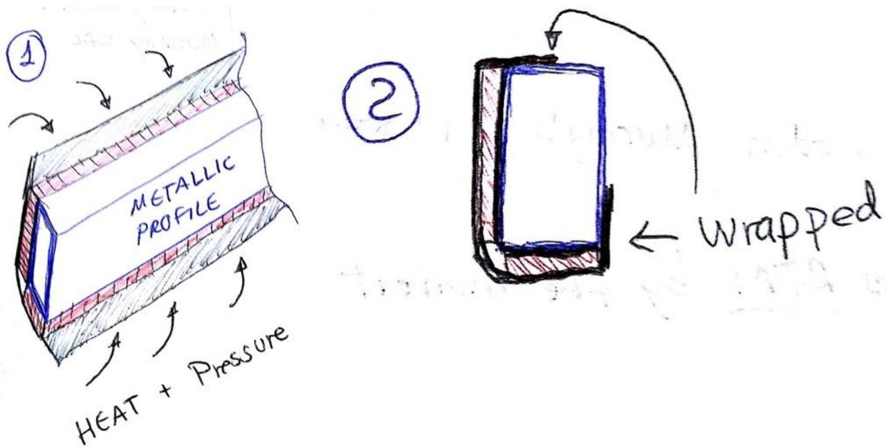
**Figure 26: wrapping of CFC panel around a tube**
