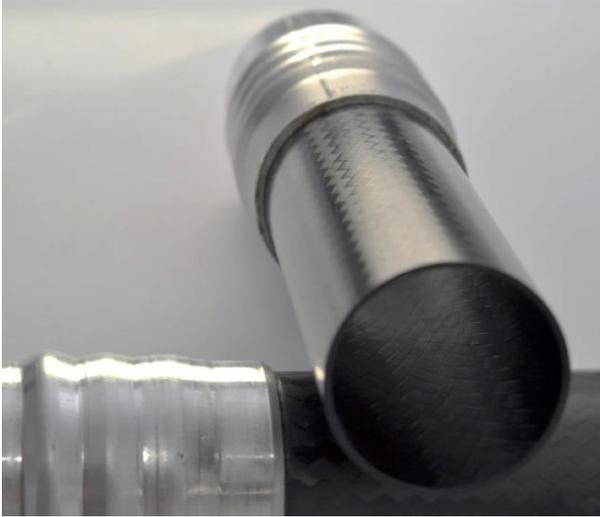
**Figure 5: TU Dresden's blow-moulding interlocked assembly**
