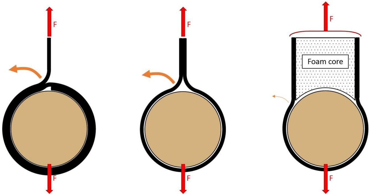
Figure 10: three configurations for wrapped joints to be further investigated. It can be expected from the third configuration to exhibit lower peeling stresses (in orange)
