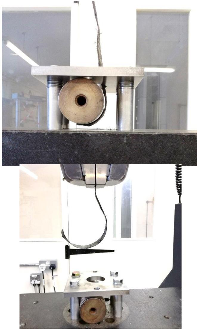
**Figure 55: on the left: the laminate is unwrapped during testing of configurations 1 to 4. On the right: it recovers a part of its original shape at the end of the test.**
