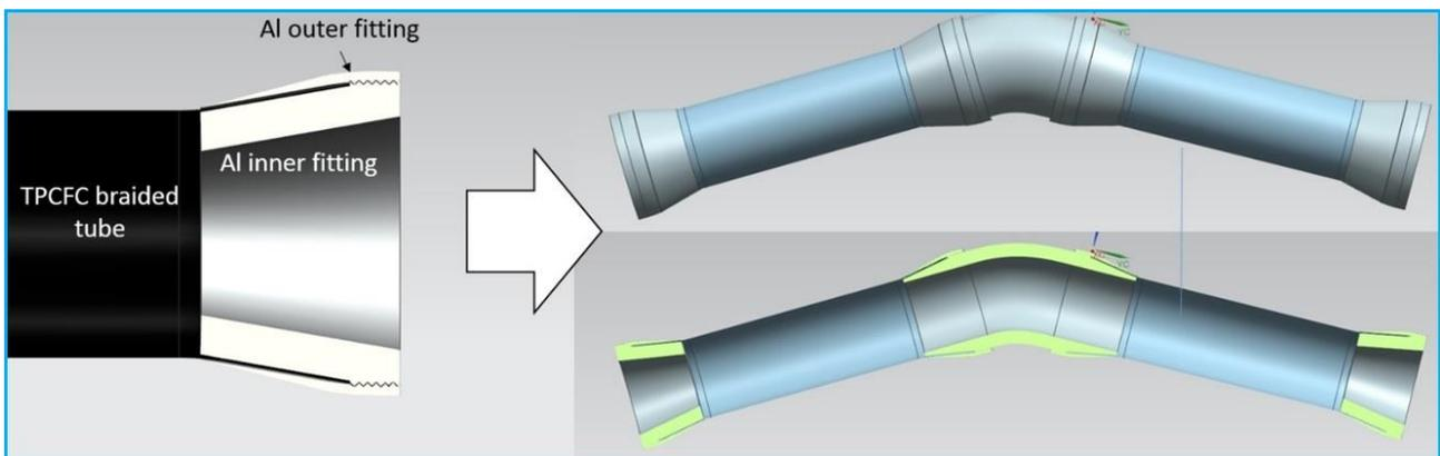
Figure 41: Concept for metal to CFC interlocking joint.
