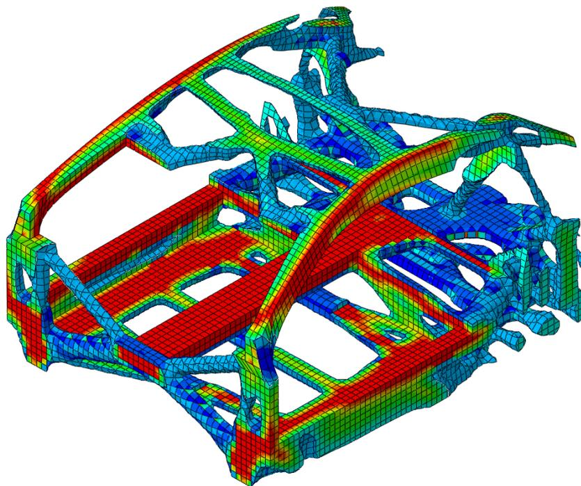
**Figure 14: topologically optimised life cell**
