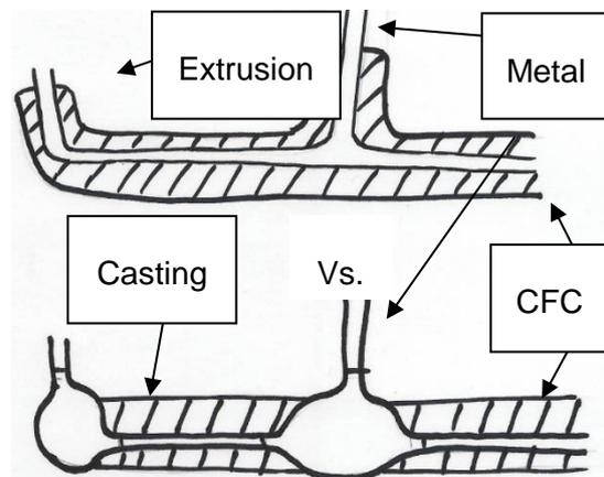
**Figure 25: Short fibre CFC to bring bulk stiffness to a thin metal skeleton**
