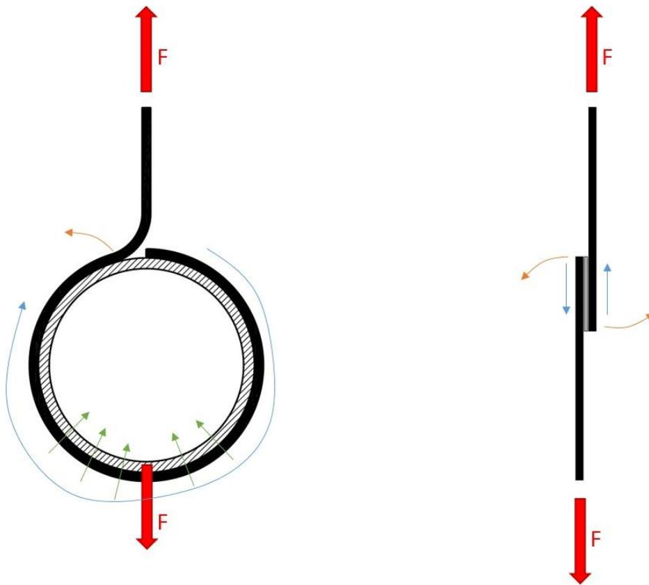
Figure 48: on left, a laminate wrapped around a tubular structure presents predominantly shear (in blue) and compression (in green), in comparison to lap shear, on the right, which presents a larger proportion of peeling (in orange)
