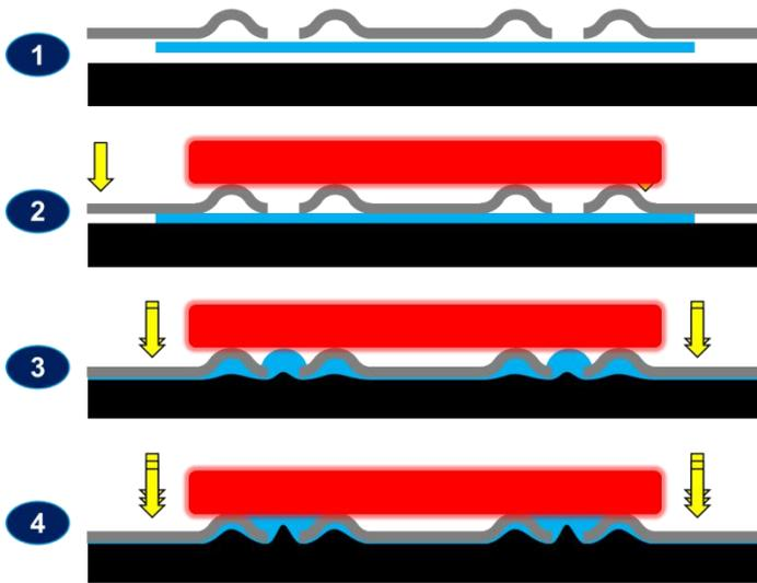
1. Assembly stack – sheet metal, weld/ bond sheet & CFRT
