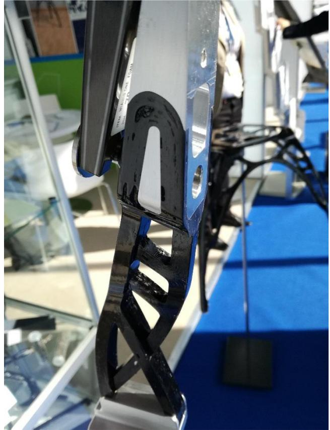
**Figure 17: seen at JEC Paris 2017, Fraunhofer's optimised frameworks are in reality made using OOA prepreg processes. However, they set an accurate design model for future 3D tow placement structures and joining.**
