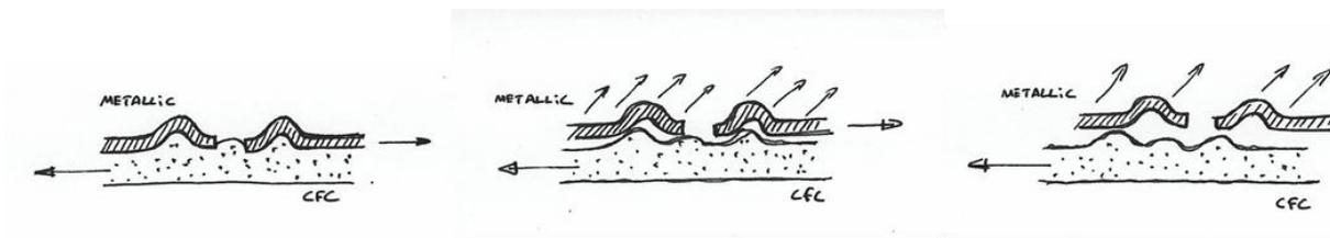
**Figure 68 - sketch of metallic plate/ CFC slipping and separation as joint loading increases**
