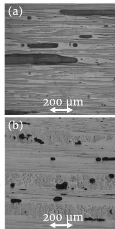
Figure 6. – Microstructure: (a) conventional; (b) LbL material.
