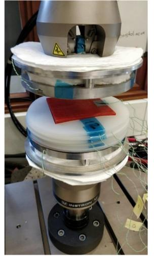
Figure 2. – Whole LbL process implementation using a servo-hydraulic machine with heated plates.
