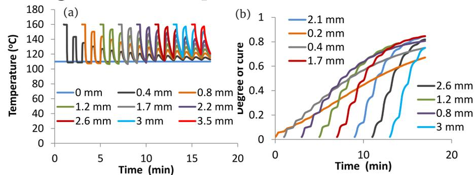
Figure 3. – Simulation of ATP LbL curing: (a) temperature; (b) degree of cure.
