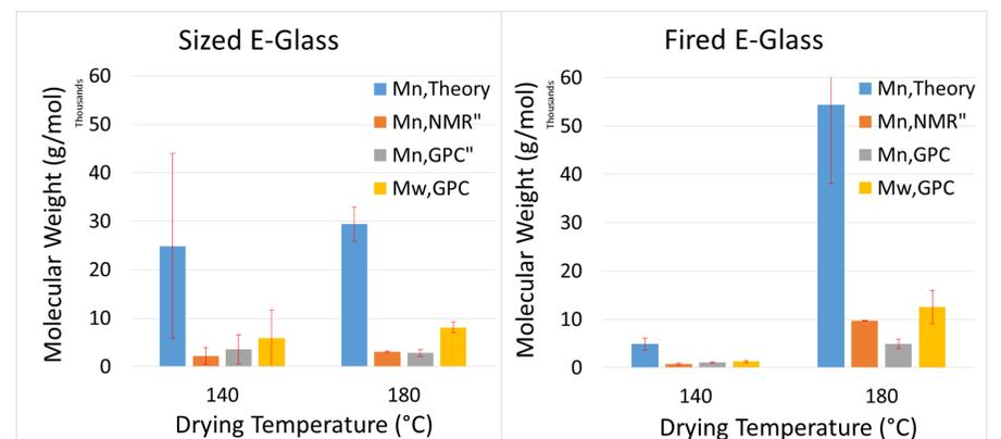
Figure.3 – Effect of fibres on the final composite molecular weight
