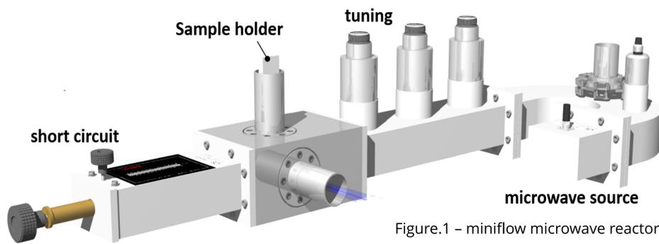
Figure.1 – miniflow microwave reactor
