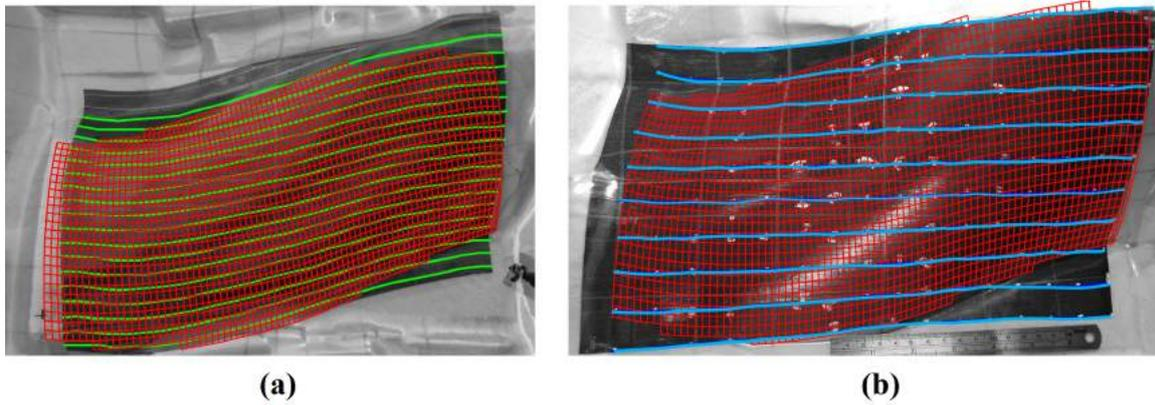
Fig. 7. (a) Comparison of finite element based projected ideal fibre path (red) and projected fibre path (green) of formed steered preform from test on twisted part; (b) comparison of finite element based projected ideal fibre path (red) and projected fibre path (cyan) on formed UD preform from test on twisted part.
