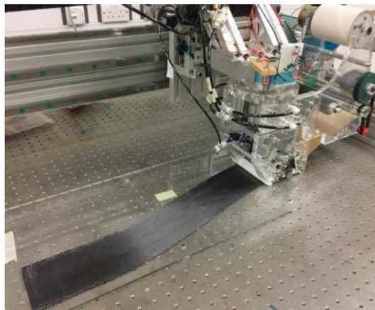
Fig. 4. Wide tape CTS machine steering a 100 mm wide unidirectional prepreg tape.
