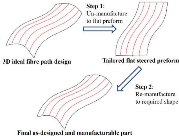
Fig. 1 Schematic of un- and re-manufacture processes in 'lay-flat and form'.
