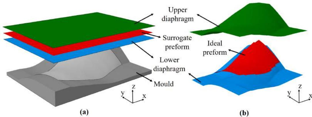
Fig.3. Illustration of (a) initial forming model, (b) unforming model. Note that diaphragms position relative to mould and preform and the size of preform are for presentation only.
