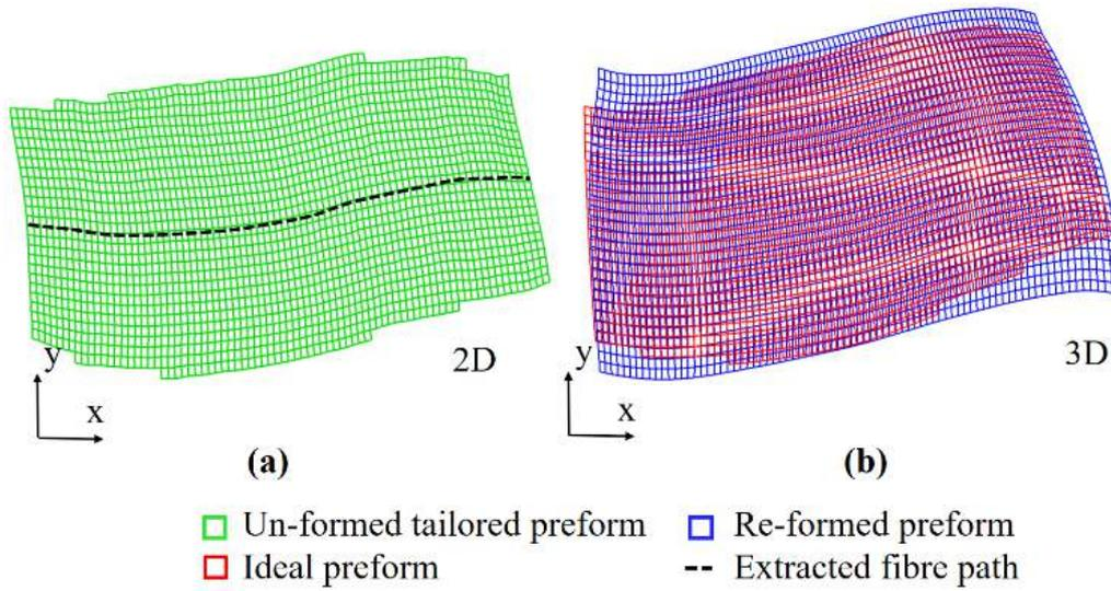
Fig. 5. (a) Un-formed preform model with extracted fibre path at mid-chord, (b) comparison of fibre path between ideal preform and re-formed preform.
