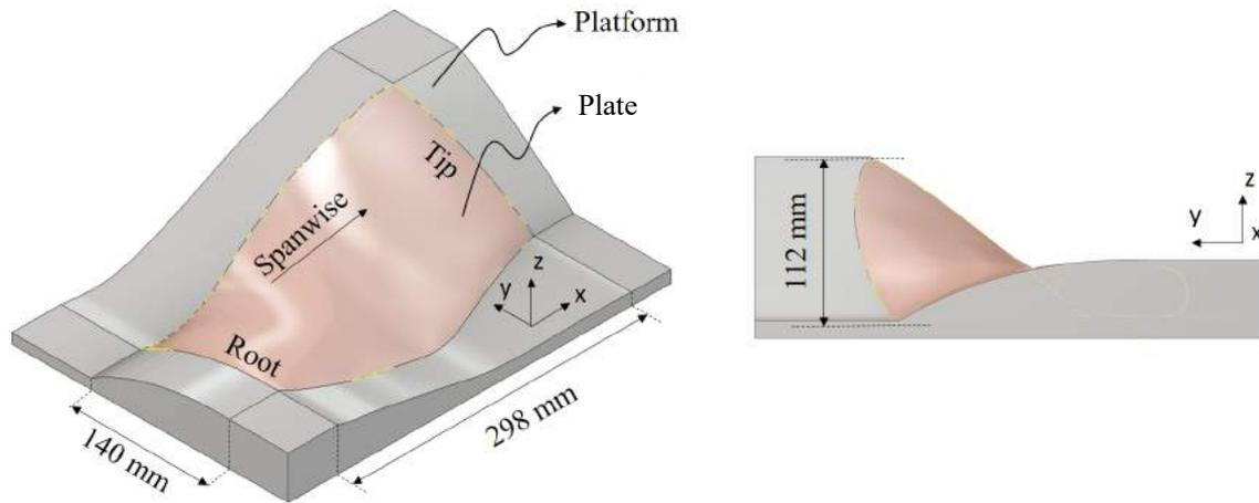
Fig. 2 Designed mould in CAD view with dimensions. The twisted plate part is highlighted in the centre of the mould
