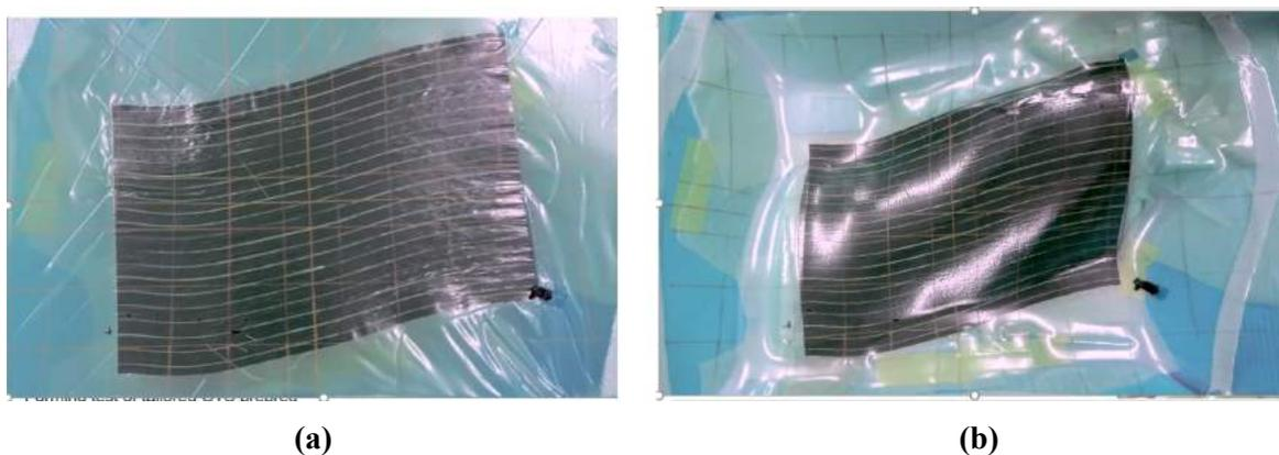
Fig. 6. (a) flat preform deposited by CTS machine; (b) CTS preform formed onto twisted part in double diaphragm forming rig.
