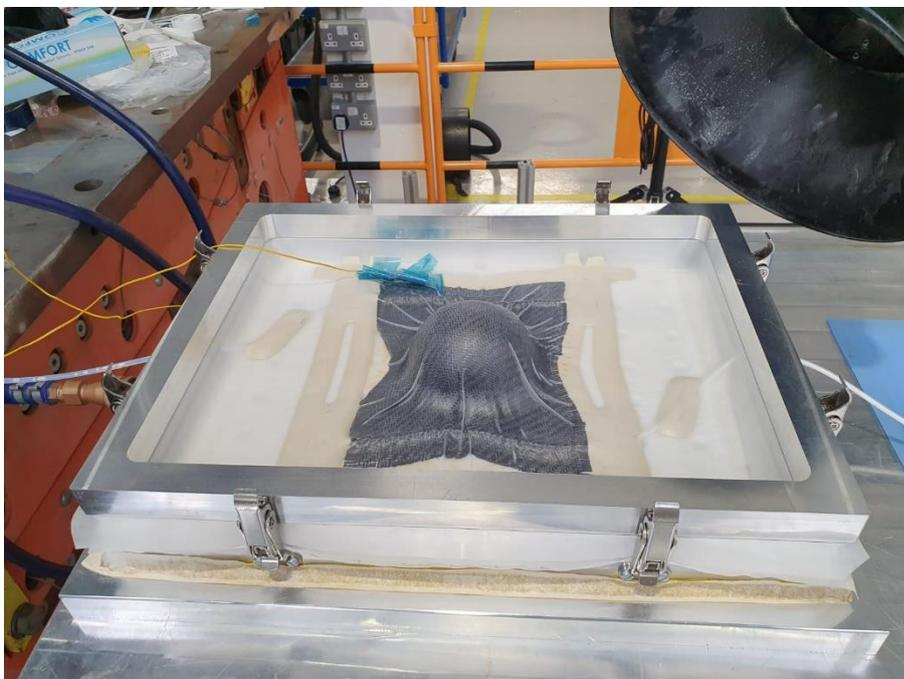
*Forming with carbon fabric, using a silicone bag*
