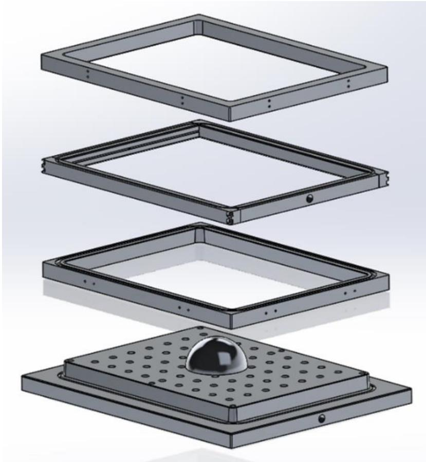
*Small scale forming frame with vacuum base and hemisphere former*
