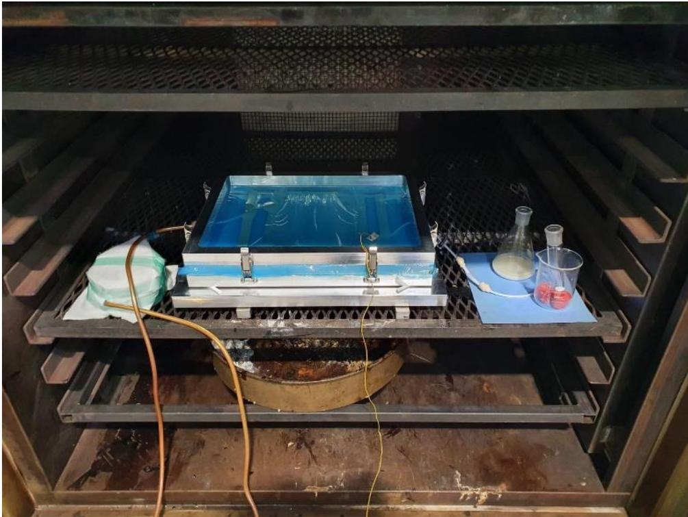
*Vacuum infusion setup in oven at UoN*
