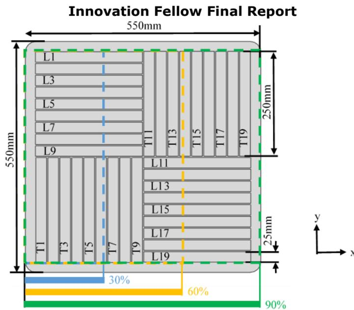
Figure 18: Schematic of the initial charge locations and tensile testing sample layout for the indirect validation study. L1-L9 are referred to as longitudinal, low flow. T1-T9 are referred to as transverse, low flow. L11-L19 are referred to as longitudinal, high flow. T11-T19 are referred to as transverse, high flow.
