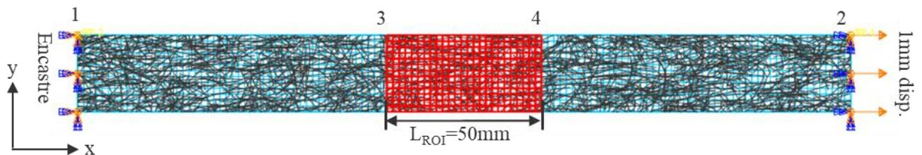
Figure 17: Example meso-scale virtual tensile testing coupon generated in ABAQUS/standard.
