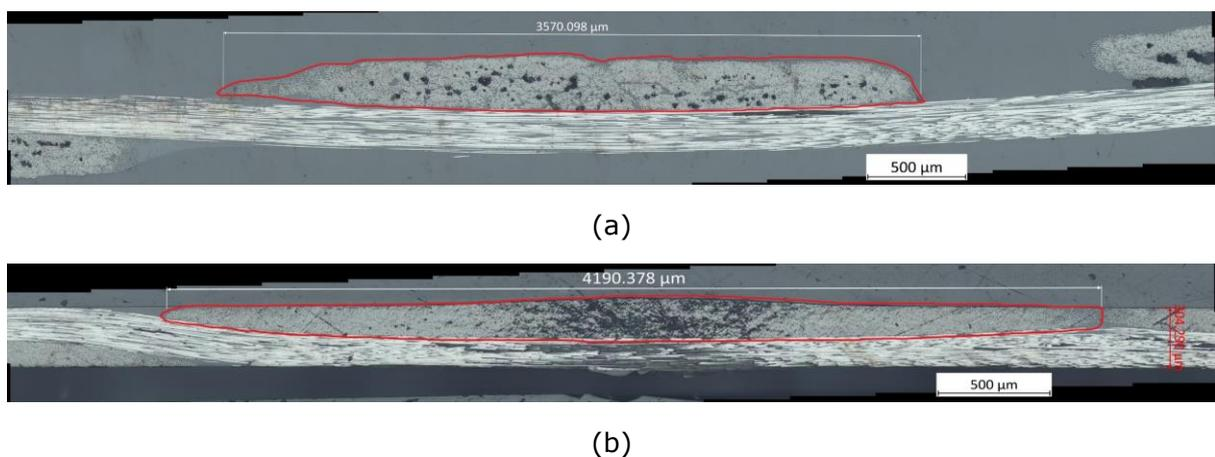
Figure 9: Micrographs showing typical cross-sectional dimensions of prepreg tows (a) before compaction and (b) after compaction.
