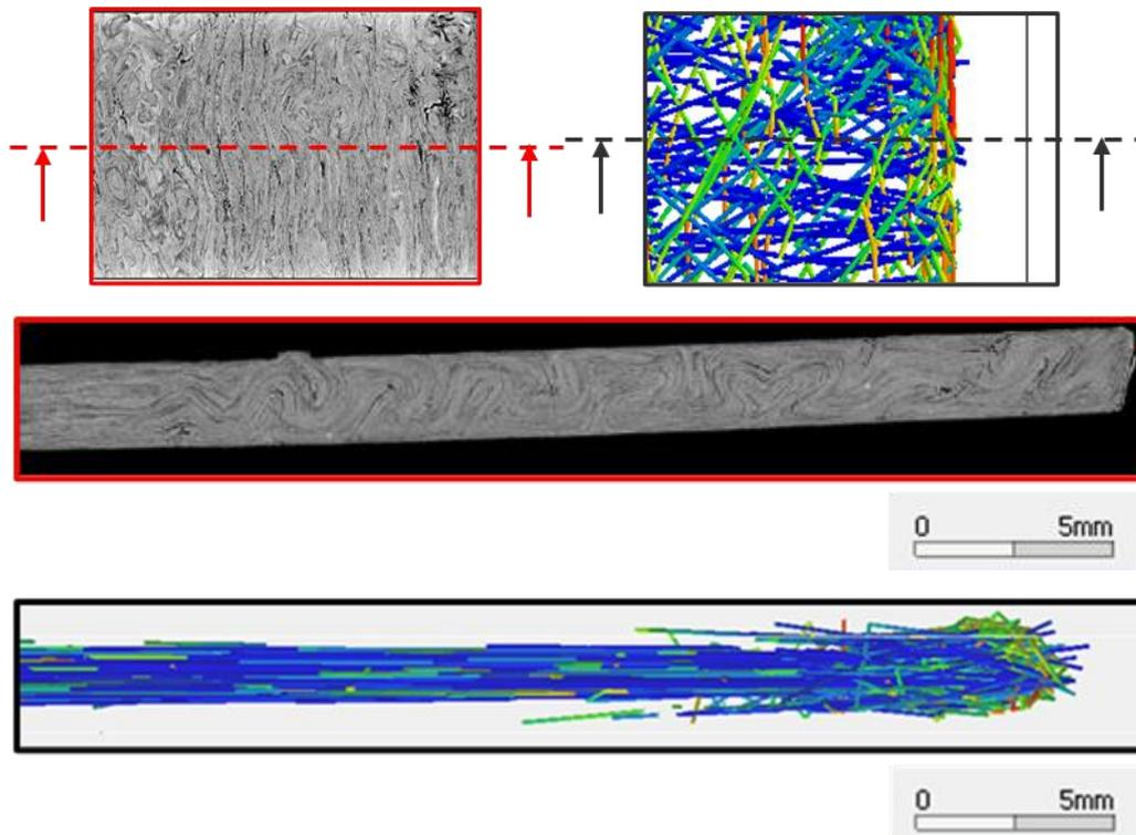
Figure 22: Meso-scale fibre architecture comparison between  $\mu$ CT scan and DFS results. The sample was indicated by the yellow box in Figure 20
