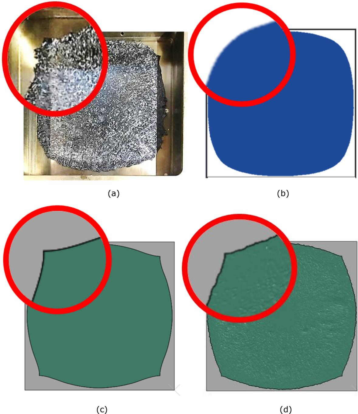
Figure 16: Filling pattern comparison for the flat plaque geometry. (a) Experimental. (b) Moldex3D. (c) Proposed new model with regular charge thickness. (d) proposed new model with irregular charge thickness.
