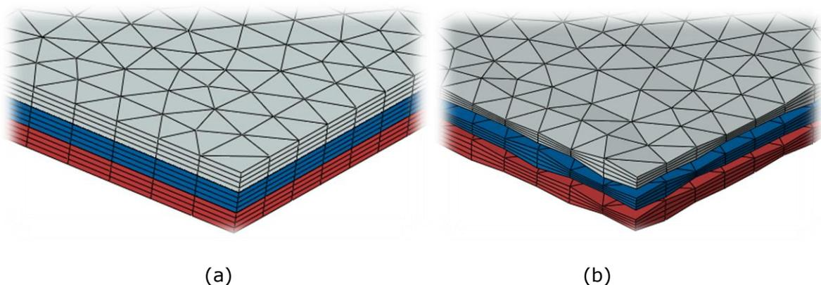
Figure 15: Initial charge modelled using (a) regular thickness approach and (b) irregular thickness approach
