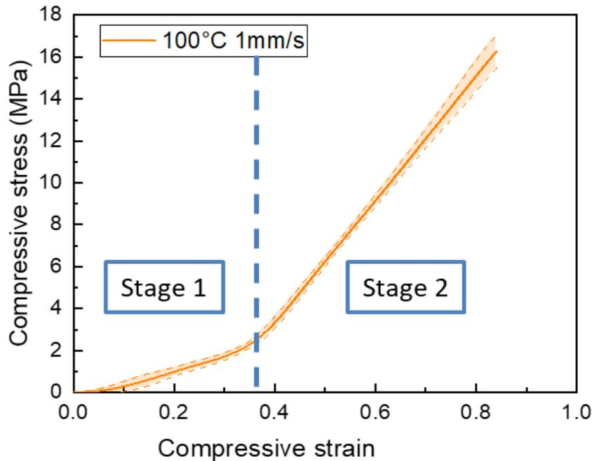
Figure 10: Compressive stress-strain curve from prepreg compaction test. The area bounded by the dashed curved indicate the variability range from seven repeat tests.
