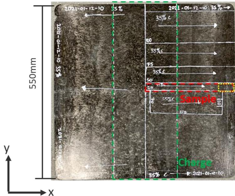
Figure 20: Schematic of the  $\mu$ CT sample location, initial charge location in relation to the flat plaque.
