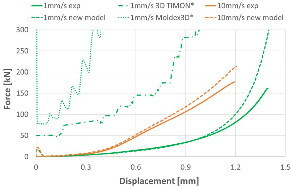
Figure 14: Comparison of force-displacement curves from the squeeze flow tests between the proposed new constitutive model, selected commercial software and the experimental data.
