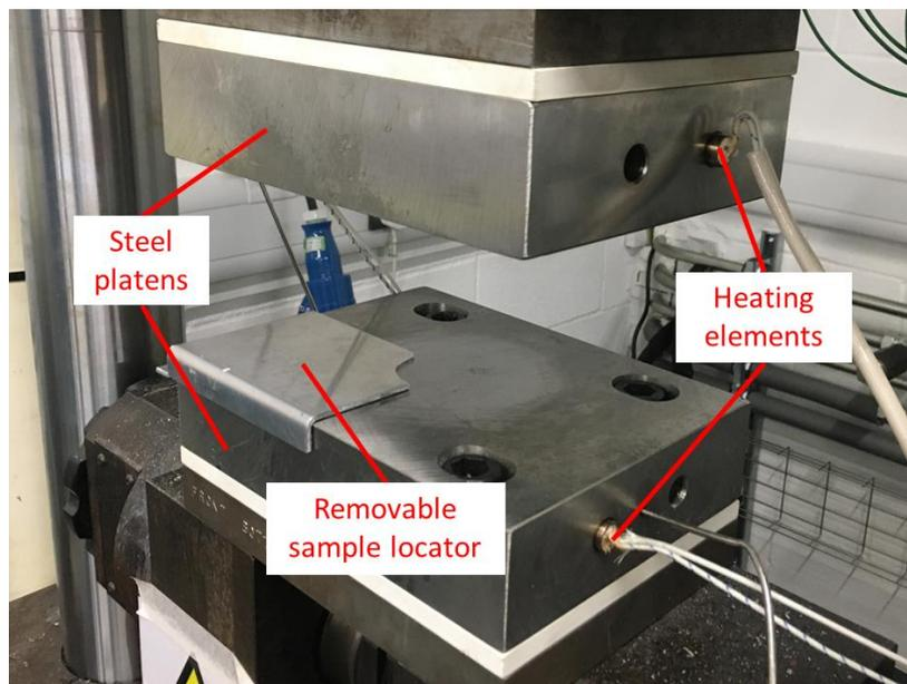
Figure 2: The old compression testing rig.
