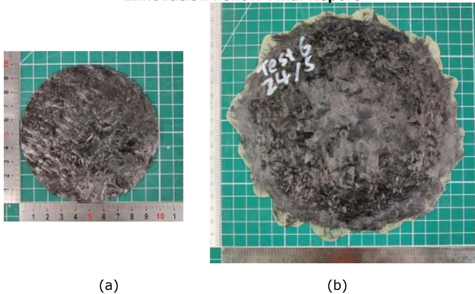
Figure 6: Comparison of an SMC squeeze flow sample (VE based, 25mm fibre length, 37%vf) (a) before test and (b) after test. The test was performed at 1mm/s closing speed and 100°C.
