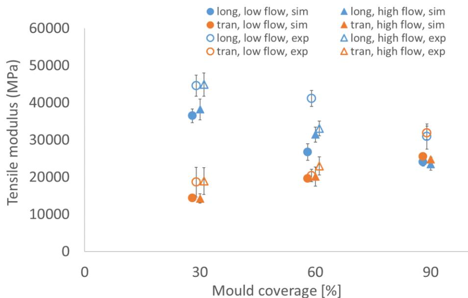
Figure 19: Comparison of tensile modulus predicted from simulation against experimental. The sample configurations are be found in Figure 18.
