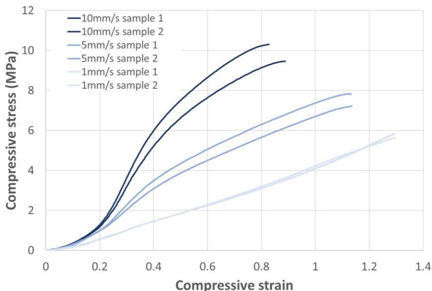
Figure 7: Compressive stress-strain curves for an example SMC material (VE based, 25mm fibre length, 37%vf) at different testing speeds and a constant testing temperature of 100°C. All samples were terminated at a 200kN force.
