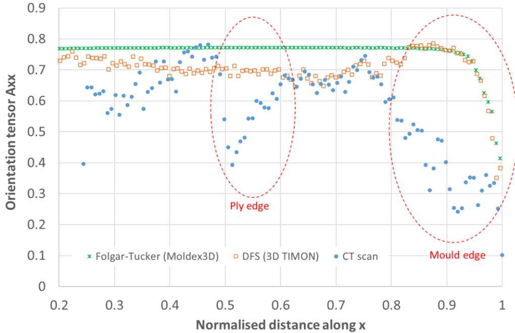
Figure 21: Comparison of fibre orientation tensor  $A_{xx}$  distributions along the sample length between the Folgar Tucker model, the DFS model and the  $\mu$ CT data.
