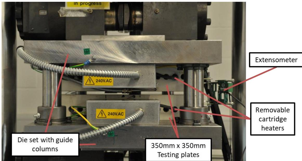
Figure 4: The new compression testing rig delivered through the project.
