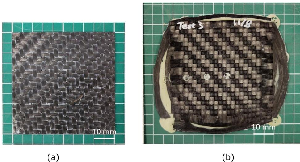
Figure 8: Comparison of prepreg compaction sample (a) before test and (b) after test.
