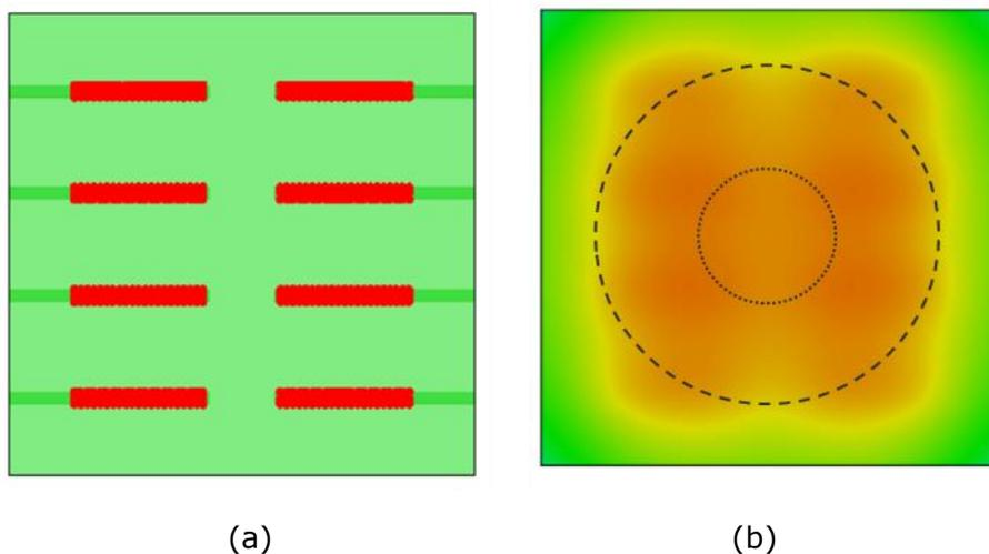
Figure 5: Optimised heating plan (a) cartridge heater layout (b) effective temperature distribution.
