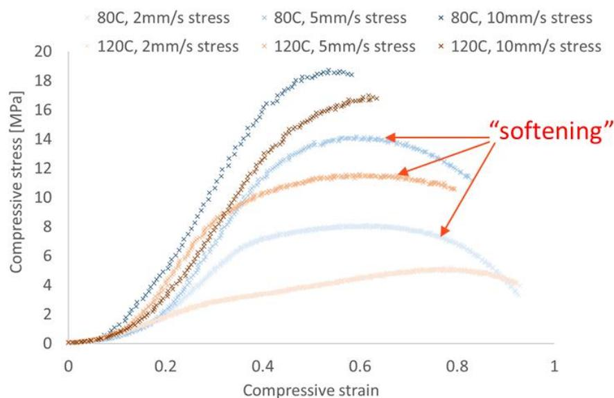
Figure 3: Typical compressive stress-strain curves from SMC squeeze flow tests using the old compression testing rig (see Figure 2)
