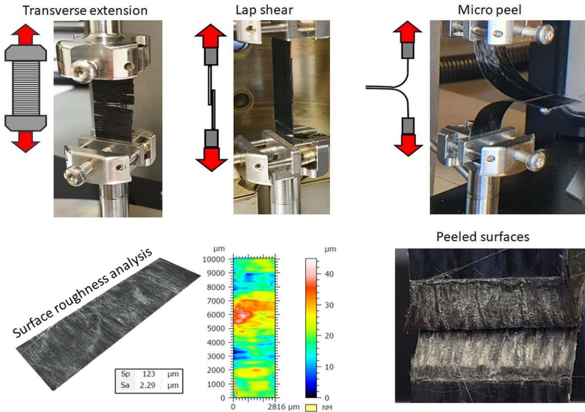
Methods employed to study the detachment of the matrix in order to peel consolidated composite plies. The surface roughness of the peeled surfaces was also recorded.
