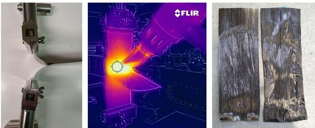
Large scale peeling of consolidated composite plies was achieved using heat and a small load. The peeled plies showed some surface disturbance but could be reprocessed into components with comparable properties to virgin plies.
