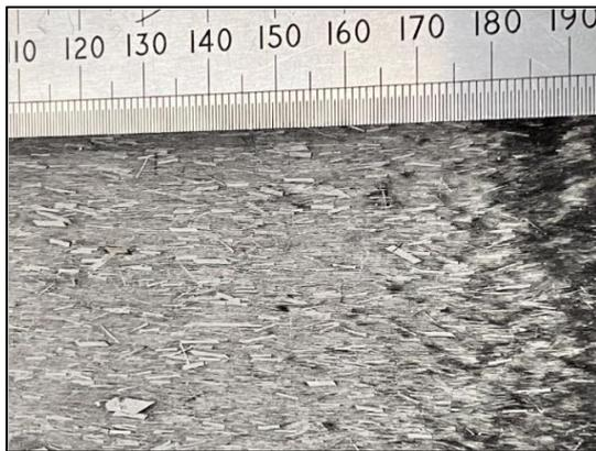
Progression of the feasibility study enabled the project scope to accommodate a trial of using carbon fibre recycled from end-of-life composites that were recovered by pyrolysis. This trial was limited to using the recycled carbon fibre in the alignment process. The image on the left shows the achieved fibre alignment. It can also be seen that fibre dispersion remains a significant challenge when end-of-life recycled fibre is used.
