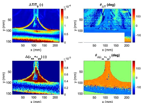
Figure 2. Normalised temperature change (TSA) and phase with respect the load applied (top) and change of strain in x and y sum (UDIC) and phase with respect to the load applied (bottom)
