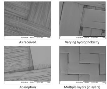
The results indicate that polymers can be selected that tend to wet-out fibre by varying amounts. This could lead to tailoring whether printed polymers acts to primarily stabilise fibrous materials or to be available on their surface to tack together plies during laminate lay-up and preform building.
