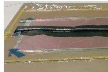
CNT dispersed in resin being infused into a glass fibre preform to determine manufacturing method of the composite
