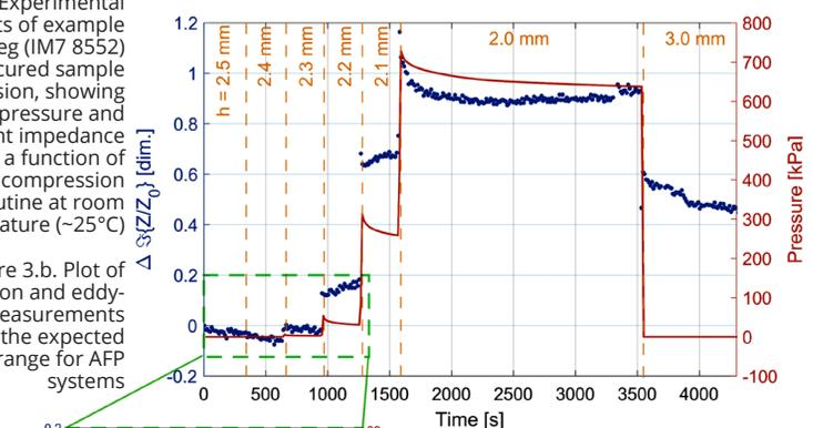
Figure 3.b. Plot of compression and eddy-current measurements within the expected pressure range for AFP systems
