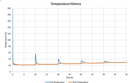
Figure 4. Thermal History Results from the Heat Transfer Model
