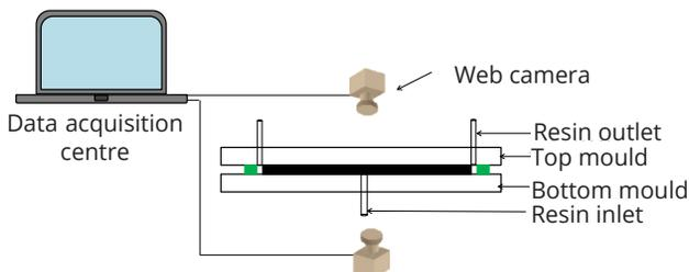
In-plane permeability of 3D woven preforms with different binder architectures- Orthogonal, Angle Interlock and Layer-to-layer is measured for Epoxy IN-2 resin and hardener mixture with a viscosity of 0.225 Pa.s
