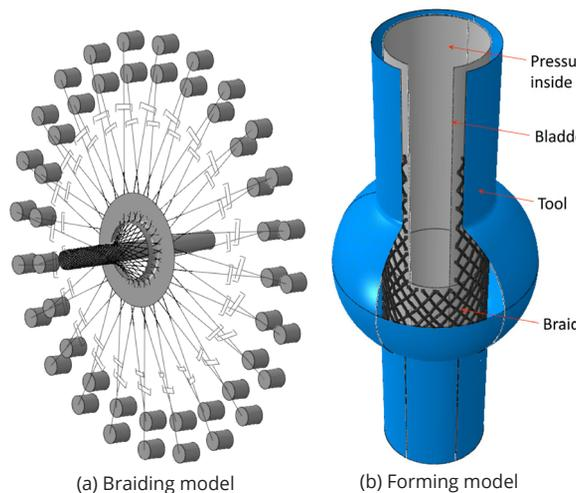
Figure 2. FE models for braid forming process
