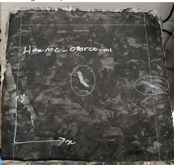
Figure 1b. Moulded Hexcel HexMC plaque showing shift of tracer tows
