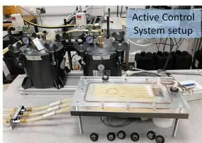
Figure 3. Active control system for RTM
