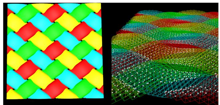
Figure 2: Current development of automated braid production in TexGen: (a) basic 2D biaxial braid (b) shows intersection points of the model.
