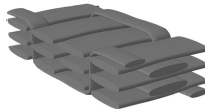
Figure 4. Nominal orthogonal weave geometry as produced from TexGen
