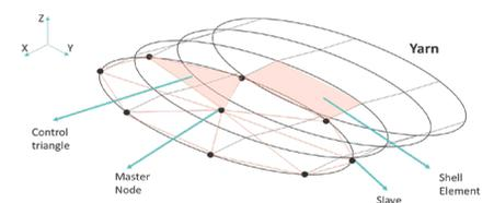
Figure 6. Schematic of hollow yarn – shell element methodology for dry fibre analysis.
