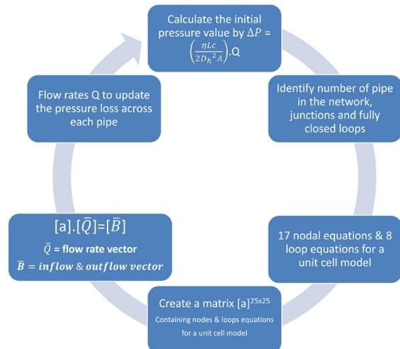
Figure3. Flow chart of the iterative process to calculate flow rates in a complex gap networking using Linear Graph Theory
