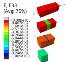
Figure 2. Material model calibration for hypo-elastic penalty contact simulation using a simple 3 element model.
