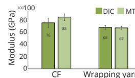
Figure 5. Tensile modulus of UD CF and CF/PP doubly wrapped yarn composite
