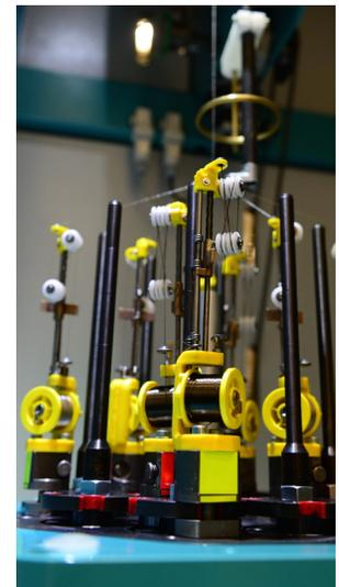
Figure 3. A Herzog 1/16 80 operates in a maypole fashion with each carrier following a specific path.
