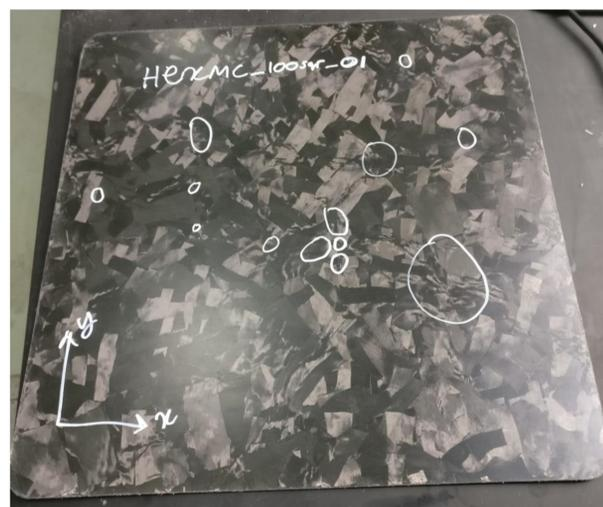
Figure 2b. top surface of 100% coverage HexMC plaque
