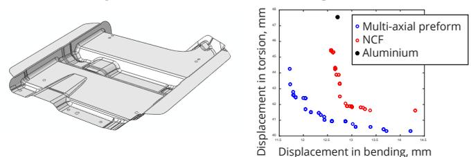
Figure 3. a. Geometry of a vehicle floor pan; b. Multi-objective optimisation of bending and torsional stiffness
