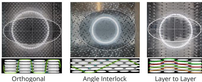
The principal in-plane permeability values K1 and K2 were determined based on least square fit technique for the elliptically shaped flow front as a function of time using the following equations which is well documented by Weitzenböck et al.[1,2]
