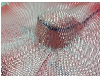
Dry woven glass fabric formed in a mould
