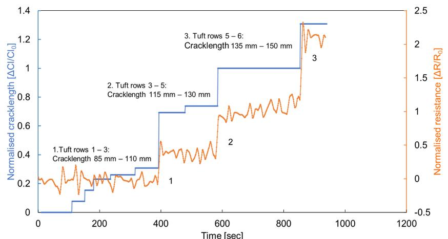
Figure 5. Tufted coupon: Crack propagation vs. electrical resistance
