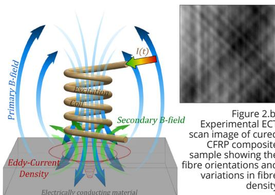
Figure 2.a. Diagram of eddy-current magnetic sensing principle showing a coil excited with alternating current, generating a varying magnetic field that induces eddy-currents in electrically conducting materials which interact with the coil.
