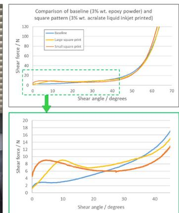
Printed polymers modify textile stiffness. Maintaining the total quantity of deposited polymer, to be common in all instances, varying printed patterns (to control the distribution of polymer) effects the stiffness to varying amounts. This effect is most pronounced within the first 20° of in-plane shear.
