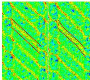
Figure 1. 0 and 0.1mm extension of NCF showing fibre bending under shear load 3D scanned
