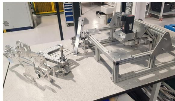
Developments of the automated dry fibre placement test rig (left) and ongoing assembly of the deposition head (right)
