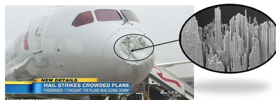
Figure 1. Boeing 787 Dreamliner's carbon fibre nose smashed in (Mail Online, 2019, Lpdlabservices.co.uk, 2019)
