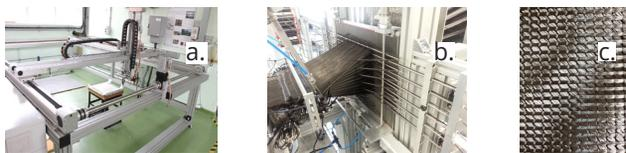
Figure 2. Multi-axial preforming (a and b); multi-axial fibre preform (c)
