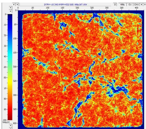
Figure 2a. C-scan of 100% coverage HexMC plaque
