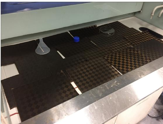
**Batch of CAGed lamina produced demonstrating scale-up of the process.**
