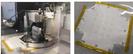
Patterns printed using research grade inkjet printers (FujiFilm Dimatix DMP2831)
