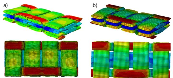
Figure 5 . Comparison of compacted geometry for a) Hypo-elastic Compliant Matrix model and b) Dry Fibre Contact Simulation.
