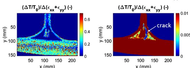
Figure 3. Damage identification by integrating TSA and UDIC at different scales
