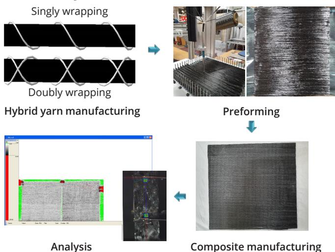
Figure 2. Composite analysis process
