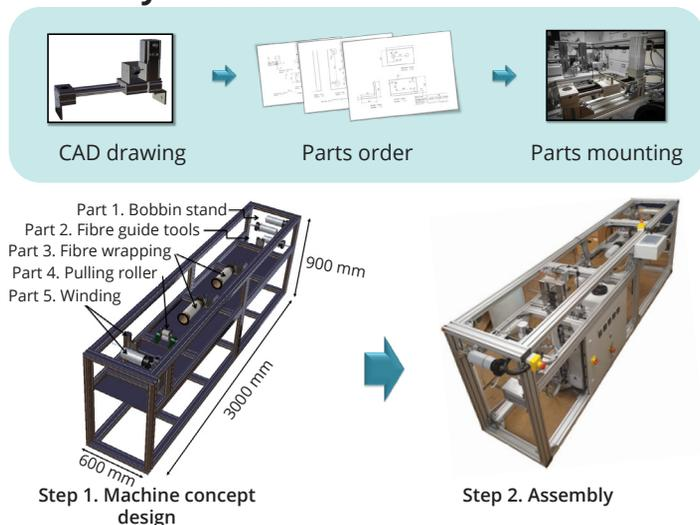
Figure 3. Development of hybrid yarn manufacturing process
