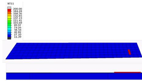
Figure 3. Element Activation Heat Transfer Model
