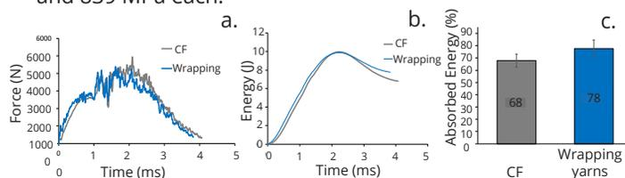
Figure 6. Force-time; (a) & energy-time history (b) of the composite samples at 10J and absorbed energy of CF and wrapping yarn composites (c)
