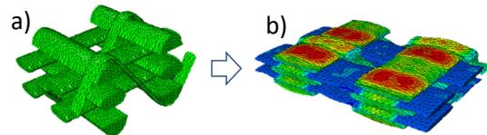
Figure 3. a) Nominal orthogonal weave mesh as generated from TexGen and b) the highly compacted yarn volumes as extracted from the hypo-elastic model.
