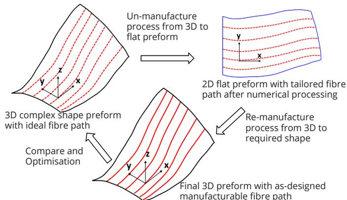
Figure 1. Schematic of the lay-flat and form
