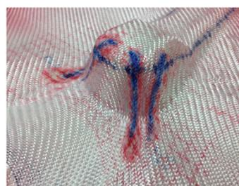
Glass fabric with stabilising resin patches
