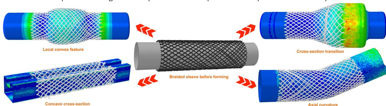
Figure 3. Formable tubular features using the proposed braid forming process
