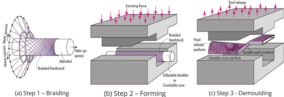
Figure 1. Preforming of complex tubular composites.
