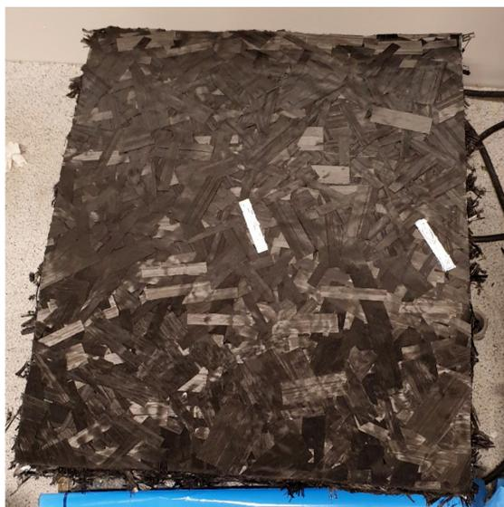
Figure 1a. Hexcel HexMC charge with tracer tows prior to moulding
