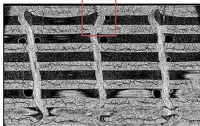
Figure 1. Binder yarn buckling and weft yarn cross-section variation in compacted orthogonal textile.
