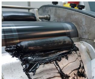
CNTs being dispersed in resin using a 3 Roll Mill to increase the electrical conductivity of the resin
