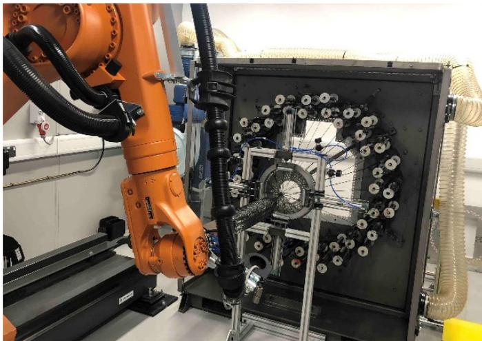
Figure 1. 48-Carrier axial braider at UoN
