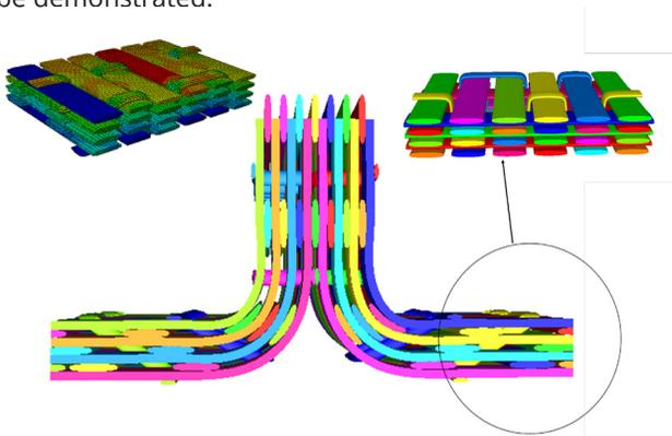
Figure 1. T-joint created using TexGen with flat flange models
