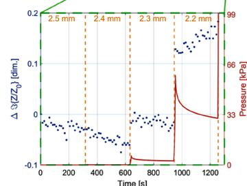
Figure 3.a. Shows the relaxation of the sample measured using ECT once pressure is removed after 3500s. This type of response will be observed behind the AFP roller head (see Figure 1)
